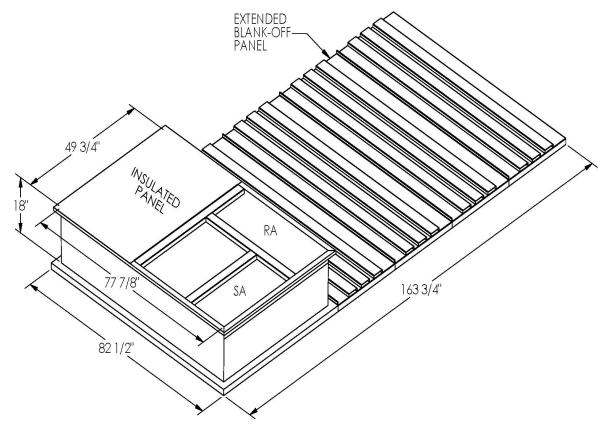
ONE PIECE WELDED CONSTRUCTION
